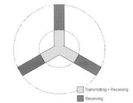
Figure 7: Repartition between transmiting and receiving antennas
