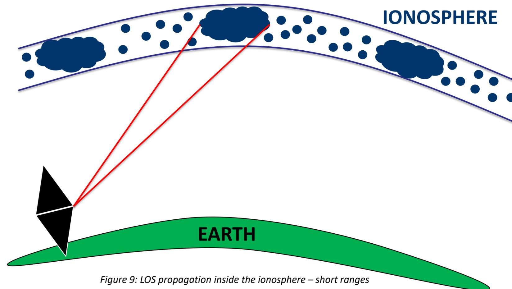
Figure 9: LOS propagation inside the ionosphere – short ranges
