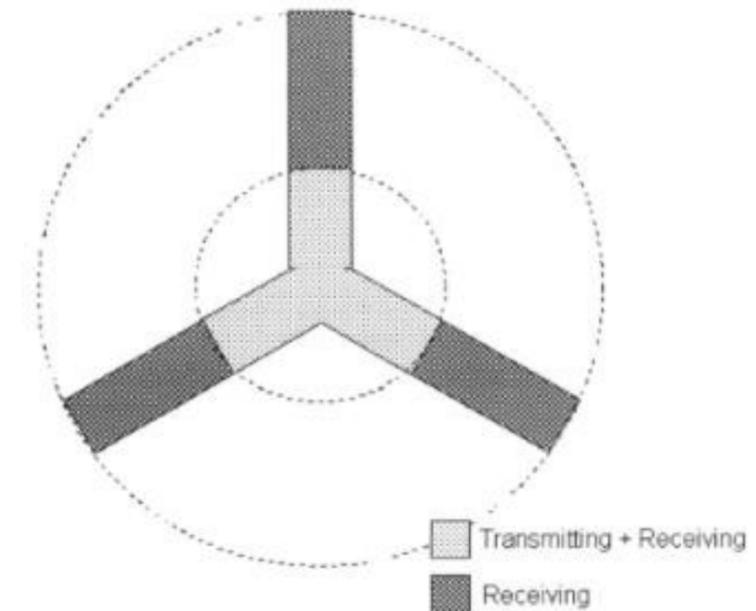
Figure 7: Repartition between transmitting and receiving antennas
